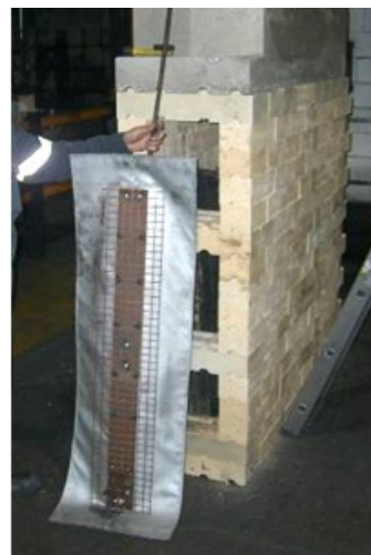
Figure 7. View of the flue wall end blanking plates (expandable baffle).
