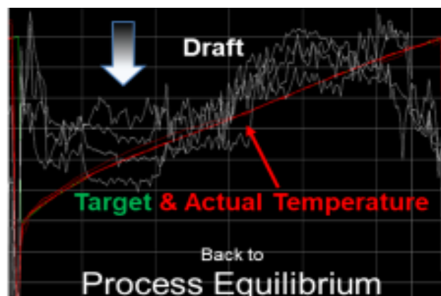
Figure 23. Back to optimized exhaust ramp temperature / draft curve – trial with optimization.
