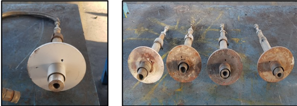
Figure 8. Comparison between new gas injector (left) and damaged ones (right).
